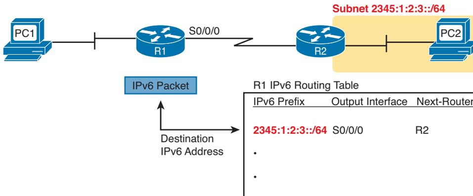
**Figure 25-6** Comparing an IPv6 Packet to R1's IPv6 Routing Table
