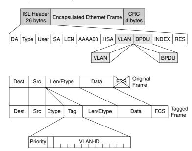
Figure 2-3 ISL and 802.1Q Frame Marking Methods
