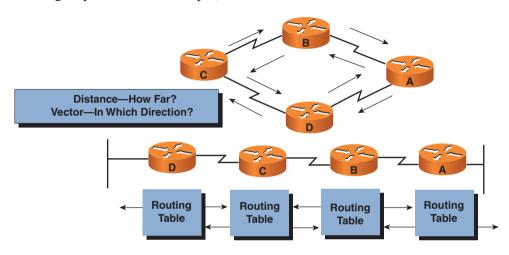
Distance accumulation keeps track of the routing distance between any two points in the network, but the routers do not know the exact topology of an internetwork.
