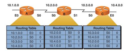
During updates, routing loops can occur if the network has inconsistent routing entries. Slow convergence on a new configuration is one cause of this phenomenon. The network is converged when all routers have consistent routing tables.
