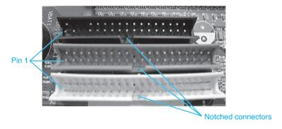
Figure 4.8 Three motherboard connectors
