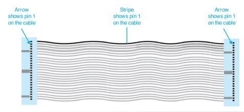
Figure 4.5 Pin 1 on a ribbon cable
