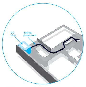
Figure 4.15 Laptop DC power plug cable
