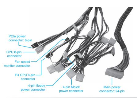
Figure 4.20 ATX power supply connectors
