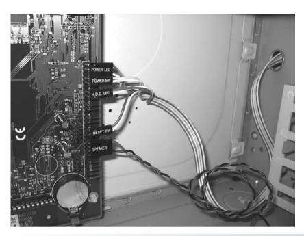
Figure 4.24 Front panel connections to a motherboard
