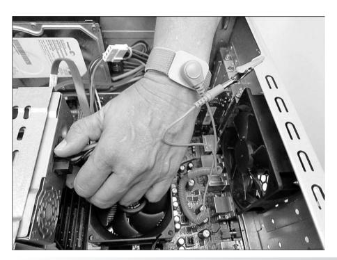
Figure 4.2 Attaching an antistatic wrist strap
