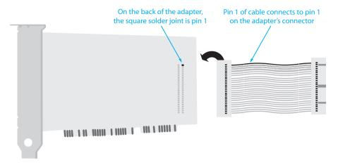
Figure 4.9 Pin 1 on a connector
