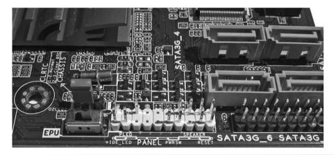
Figure 4.10 Motherboard front panel connectors
