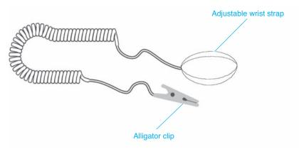
Figure 4.1 Antistatic wrist strap
