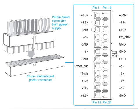
Figure 4.21 ATX 24- and 20-pin motherboard connectivity
