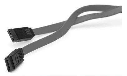
Figure 4.3 Both cable ends are the same
