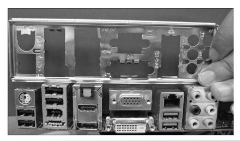
Figure 4.11 Motherboard I/O shield
