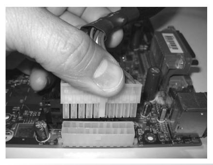
Figure 4.26 Installing an ATX power connector on a motherboard
