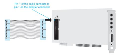
Figure 4.6 Pin 1 on an adapter
