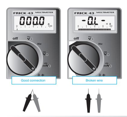
Figure 4.18 Sample resistance meter readings
