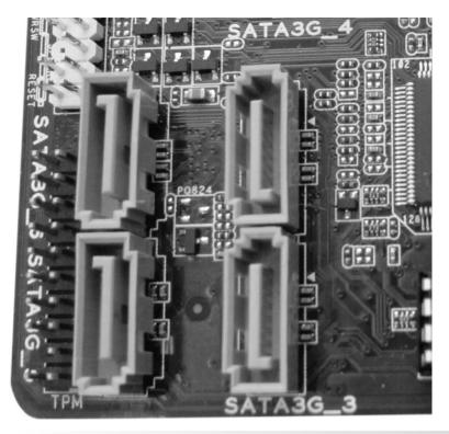
Figure 4.7 Motherboard connectors for narrow cables
