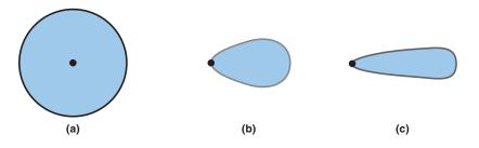
**FIGURE 4-27** Antenna radiation patterns for (a) omnidirectional, (b) Yagi, and (c) dish [parabolic reflector] antennas. The cost of the Yagi antenna is comparable to that of the omnidirectional antenna.
