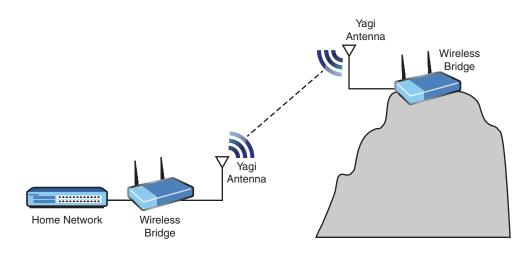
**FIGURE 4-26** The proposed point-to-point wireless link between the home network and the antenna site.
