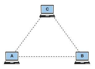
**FIGURE 4-1** An example of an independent basic service set, or ad hoc, network.
