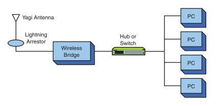
**FIGURE 4-30** The setup for the remote users in the proposed point-to-multipoint wireless network.
