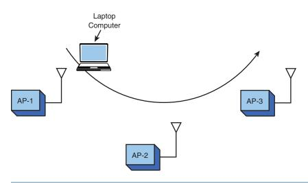
FIGURE 4-3 An example of an extended service set used for increased user mobility.
