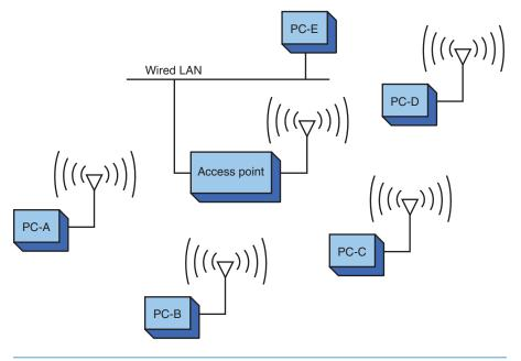
FIGURE 4-2 Adding an access point to a basic service set.
