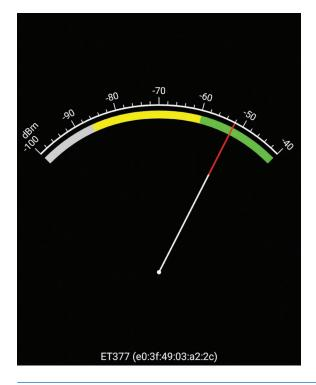
**FIGURE 4-15** The RF signal strength at point B.
