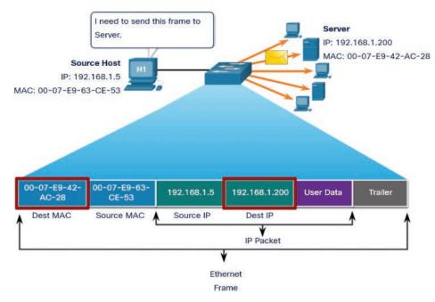
Figure 7-11 Unicast Frame Transmission
