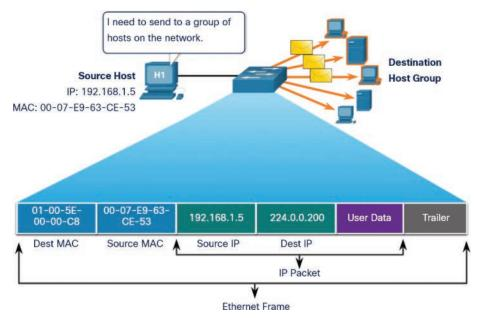
Figure 7-13 Multicast Frame Transmission
