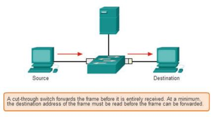
Figure 7-21 Cut-Through Switching
