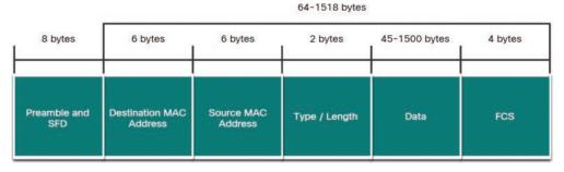
Figure 7-4 Ethernet Frame Structure and Field Size
