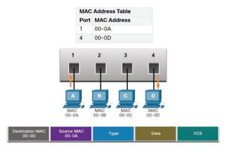
1. The switch receives another frame from PC-A and refreshes the timer for the MAC address entry for port 1.
