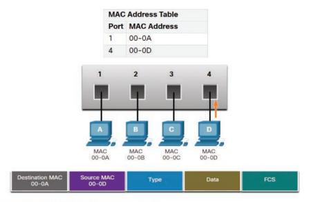
The switch adds the port number and MAC address for PC-D to its MAC address table.
