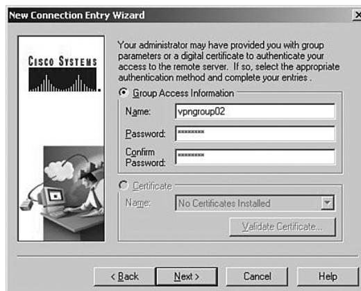
The group name that you established earlier was **vpngroup02**. Enter that in the Name field and the associated password into the Password and Confirm Password fields. The password for the IPSec group is the preshared key for the IPSec connection authentication. Click **Next** to continue.
