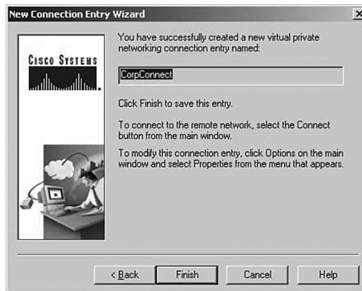
Clicking **Finish** returns you to the main VPN Client window, shown in Figure 4-42. Notice that CorpConnect now shows in the Connection Entry window and the IP address of the remote server shows in the lower window. Also notice that the **Connect** button is now active.
