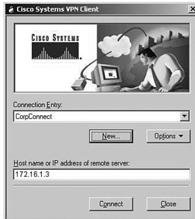
To connect to the VPN 3000 Concentrator, simply click the **Connect** button. The client attempts to negotiate IKE and IPsec SAs with the concentrator. If that is successful, the IPsec tunnel is created and the client prompts you for your username and password. Once that has been authenticated, you can begin using the VPN Client for secure remote access to the VPN concentrator.
