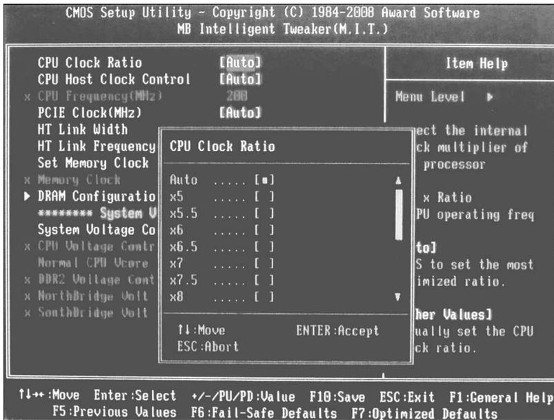
**Figure 3-22** Preparing to overclock a system running an AMD Athlon 64 X2 processor.
