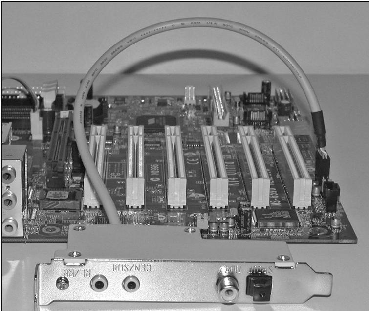
**Figure 3-6** This header cable provides support for 5.1 surround analog audio and digital audio.
