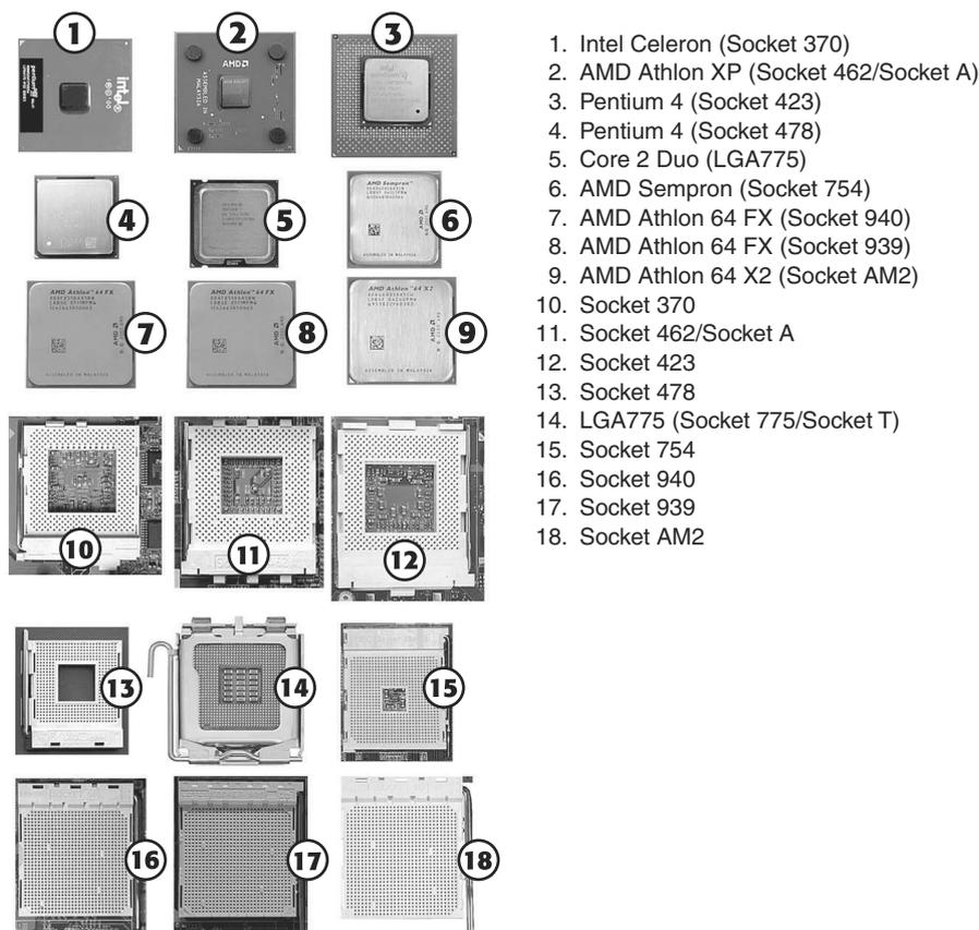
**Figure 3-21** Intel and AMD processors and sockets.
