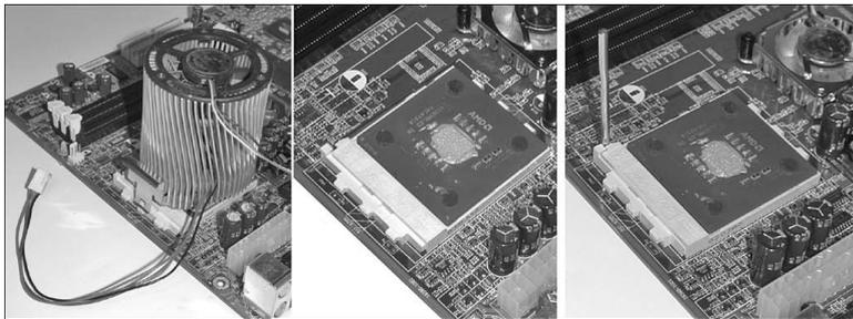
**Figure 3-28** After the heat sink fan is disconnected from power (left) to reveal the processor (center), the lever on the ZIF socket (right) can be lifted to release the processor.
