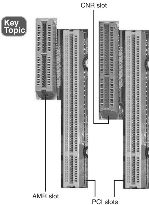
**Figure 3-10** An AMR slot and PCI slot (left) compared to a CNR slot and PCI slot (right).
