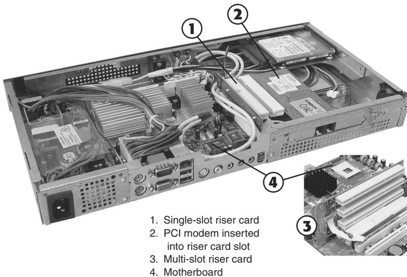
**Figure 3-4** Examples of single-slot and multi-slot riser cards.
