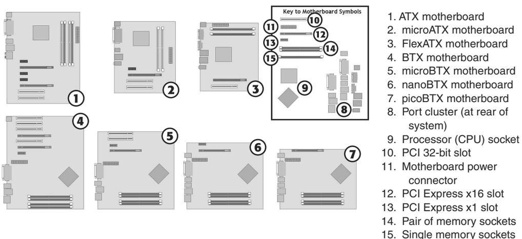
**Figure 3-2** The ATX motherboard family includes ATX (largest), microATX, and flexATX (smallest). The BTX motherboard family includes BTX, microBTX, nanoBTX, and picoBTX (smallest).
