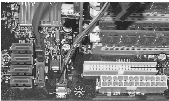
**Figure 3-12** PATA and SATA host adapters on a typical motherboard.
