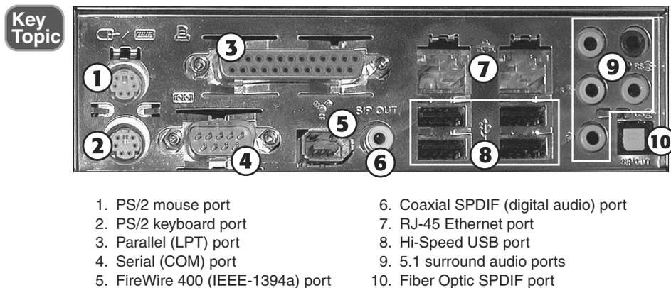
**Figure 3-5** A port cluster on a late-model ATX system.
