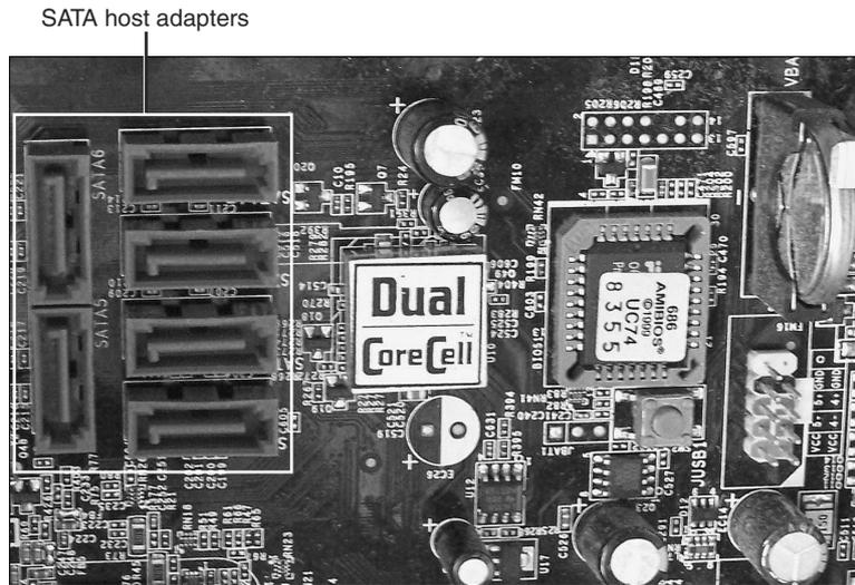
**Figure 3-13** Most late model systems include multiple SATA host adapters with skirted connectors.
