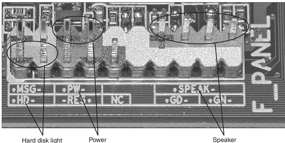
**Figure 3-18** A typical two-row front panel connector on a motherboard.
