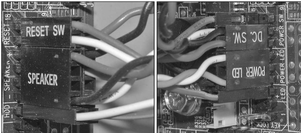
**Figure 3-15** Front-panel cables attached to a typical motherboard, which control system power to the motherboard, case speaker, drive and power lights, and so on.
