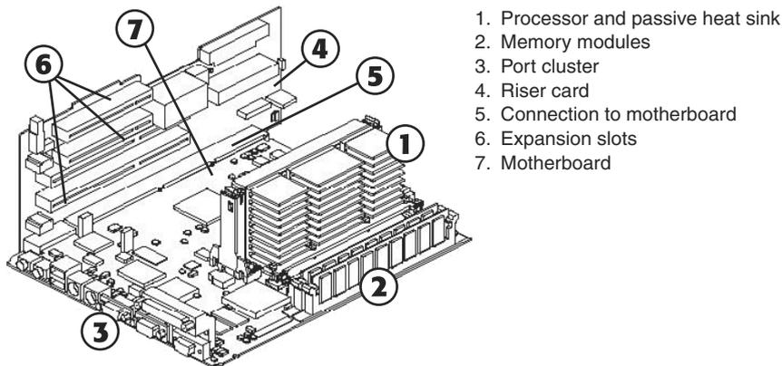
**Figure 3-3** A typical NLX motherboard and riser card.
