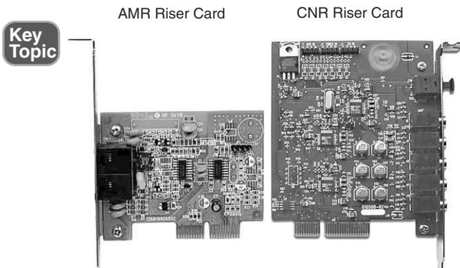
**Figure 3-11** An AMR riser card used for soft modem support (left) and a CNR riser card used for six-channel (5.1) analog and digital audio support (right).
