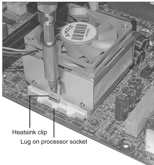
**Figure 3-24** Releasing the spring clip on a Socket A processor's heat sink.
