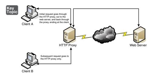
Figure 8-4 Illustration of an HTTP Proxy in Action
