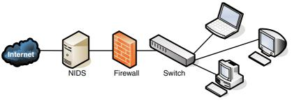
Figure 8-5 Illustration of NIDS Placement in a Network
