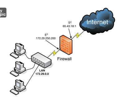
Figure 8-1 Diagram of a Basic Firewall Implementation
