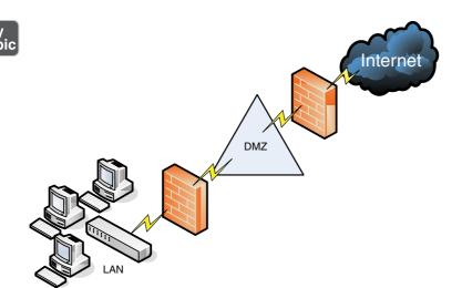
Figure 8-2 Back-to-Back Firewall/DMZ Configuration
